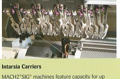
MACH2\*SIG\* machines feature capacity for up to 40 intarsia carriers. The new intarsia carriers are more compact, fitting more carriers and thus allowing more color changes within a given knitting width. The improved intarsia system is also much quieter, averaging two-thirds (2/3) less noise than our previous intarsia system.
